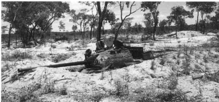
T-55 of 59 Bde. knocked out on 14 February 1988 by an Olifant of F Sqn., School of Armour; the APFSDS projectile penetrated the sand berm in front of the Angolan tank and entered the turret above and right of the gunner's sight.
