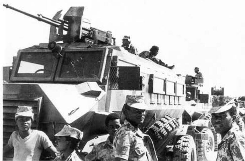
This Casspir mounts a captured 14.5mm HMG; other 'fits' included the 20mm cannon from a Vampire jet fighter, and Yugoslav 20mm cannon stripped from captured M-55 triple mounts. This photo was taken at a 'Koevoet' base; note the neat camouflage uniforms complete with rank chevrons, Police cap badges, and caps with fold-up neck flaps.
